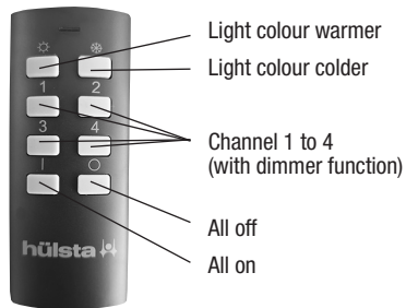
4-channel radio remote control with change of color temperature
